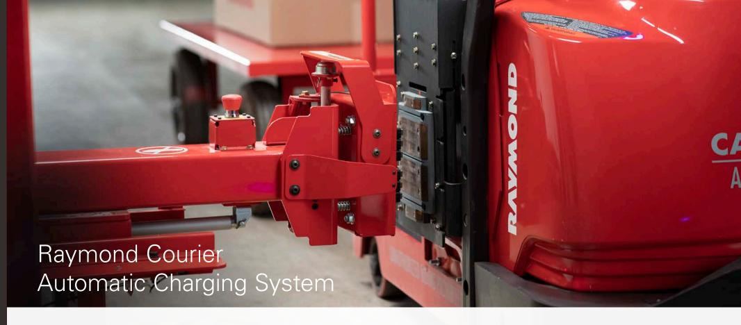
The Raymond Courier Automatic Charging System allows all Raymond Courier AGV models to automatically dispatch to a charging station, charge the battery, and return to work—even when towing or carrying a load—for 24/7 automated operation and even greater reliability, productivity, and labor efficiency.
